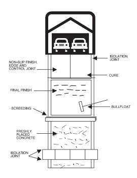
DO NOT ALLOW power floats or trowels to be used. Overworking the fresh concrete causes scaling. This extra finishing is not required and will reduce the durability of the slab.
